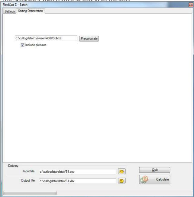
**Include pictures** – ich checked then into output file also will be included picture with sawing pattern for each log. It makes size of output file several times bigger and also calculation takes more time, because of generation of pictures.
